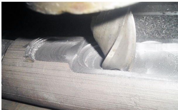
Fig. 2. View of the processing zone of the work piece with a stepped control signal
