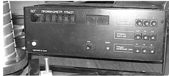
Fig. 10. Profilometer for measuring surface roughness: setting (a) and measuring part (b)
